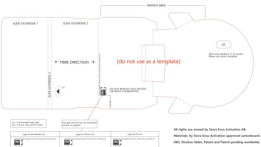
DBS logo and patent text must be printed in position shown on diagram.
